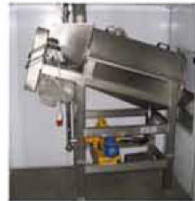
Stones cleaner with transfer pump for the recovered pulp
